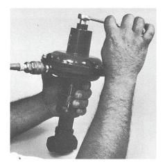
Figure 8: Adjust the valve stroke
