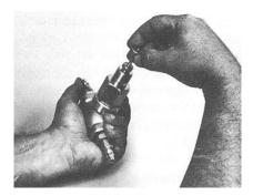
Figure 6: Lap the seating surfaces
