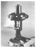
Figure 1: Separate body and bonnet from topworks
