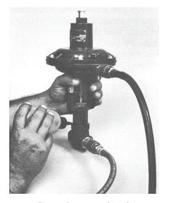
Figure 9: Pressure test the seals
