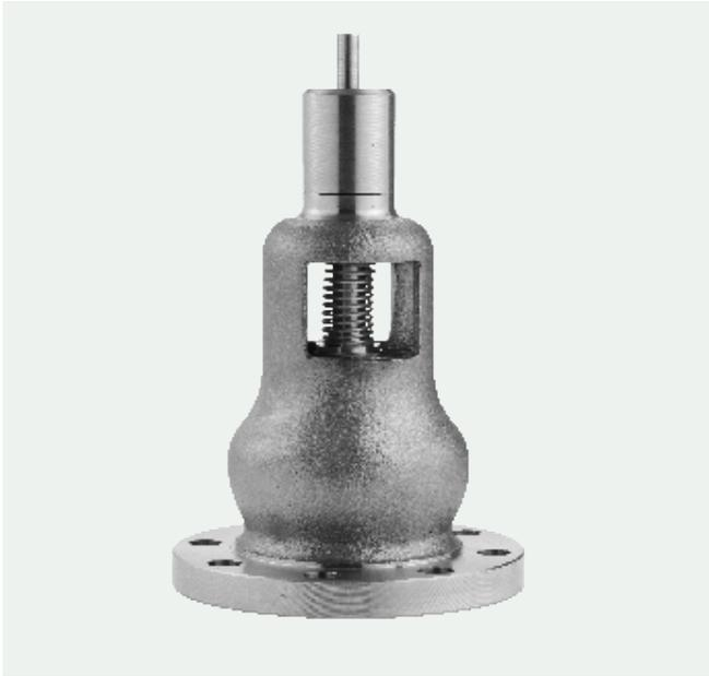
Ramén type VAC100 is a vacuum valve for protection of pressure vessels, tanks, containers, silos, hoppers, piping and other designs that may be exposed to under pressure (by media, cleaning processes, thermal variations, etc). The VAC100 will open automatically when the pressure of gases or vapors goes below 0,85-0,9 bar(a) (can be ordered with other set pressure on request) giving the construction a robust and trusted protection against vacuum that can cause unreparable damage to any system.
