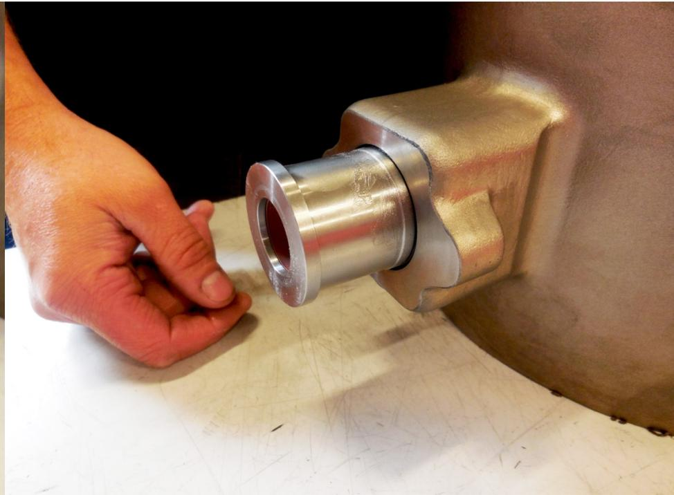
Insert the bearing sleeve (KS-4). Be careful not to damage the O-ring passing the threaded hole in the body. Push the sleeves firmly all the way in.
