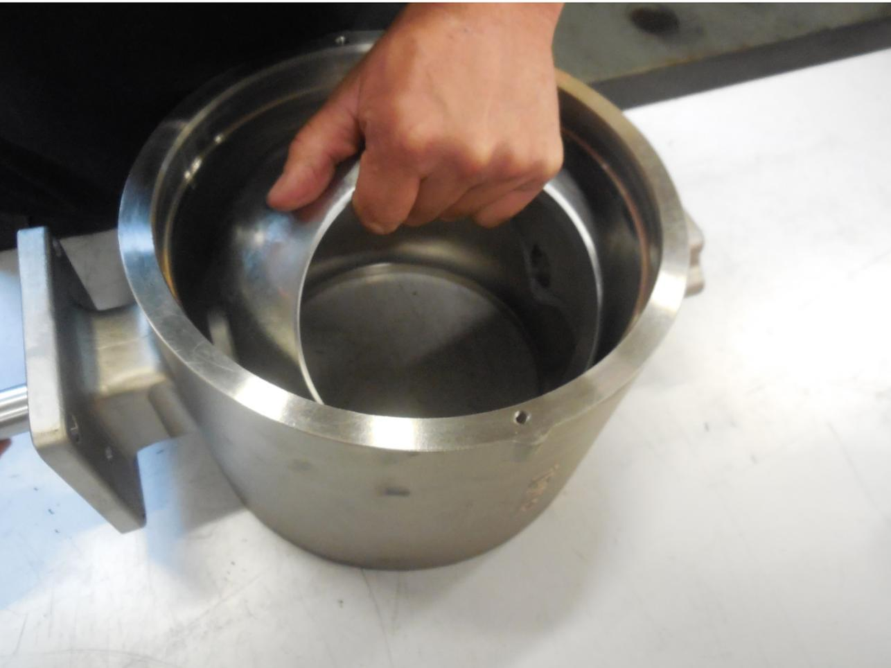
Keep the ball sector in an open position when assembling. Put the long shaft at the actuator side of the valve to your right and the ball sector as shown in the picture.
