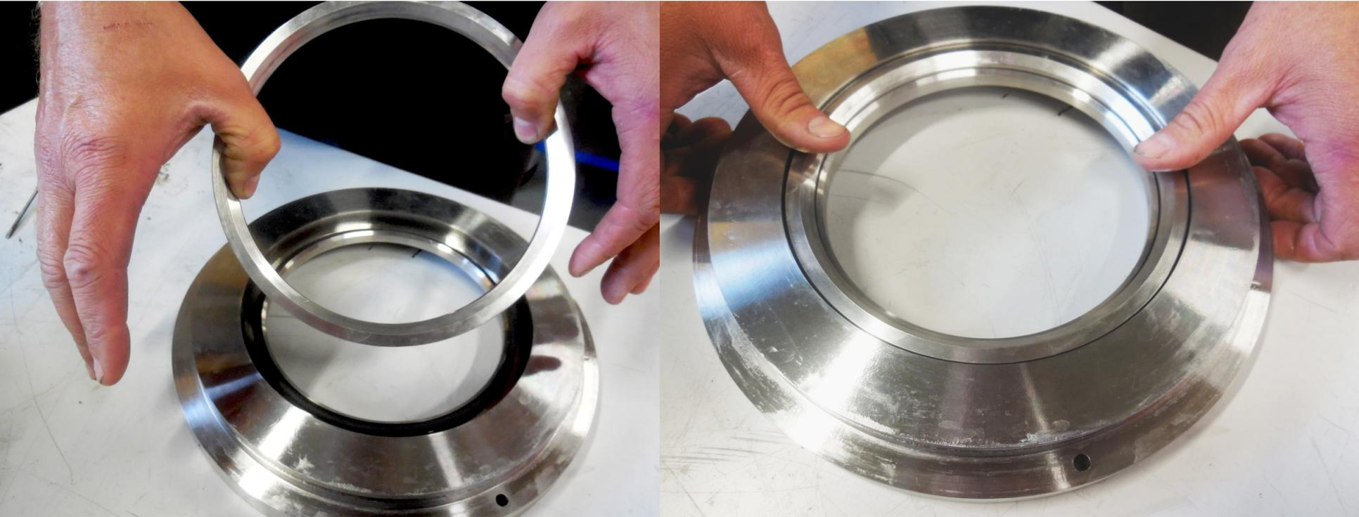
Carefully take the seat (KS-10) and press down over the O-ring (KS-15). This picture demonstrates a stellited seat, type 1B. However the procedure is the same, regardless of what kind of seat is used.
