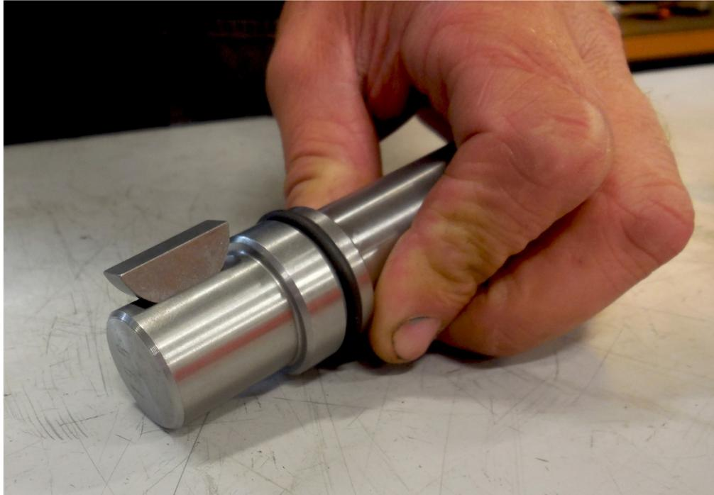
Mount the woodruff key (KS-8) in the groove, as shown in the picture. Use a rubber hammer if necessary.
