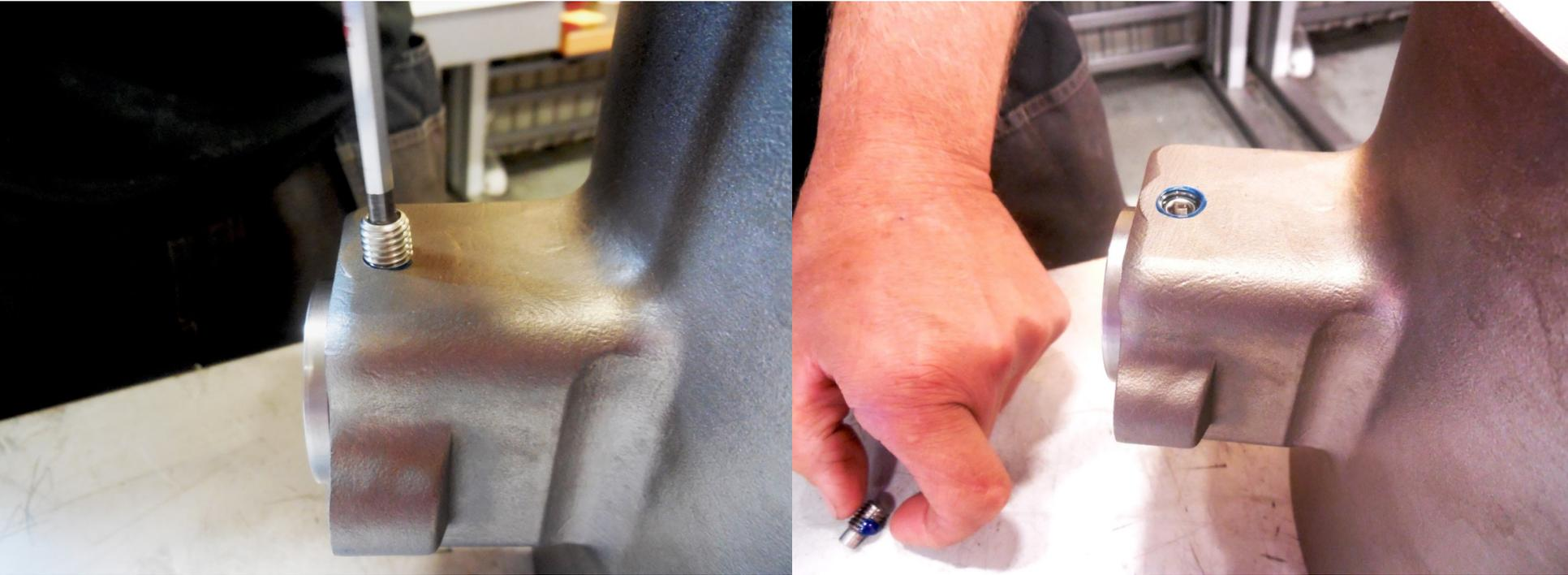
Assembly the grub screws (KS-12). Turn them clockwise all the way down and then in the opposite direction  $\frac{1}{2}$  turn.
