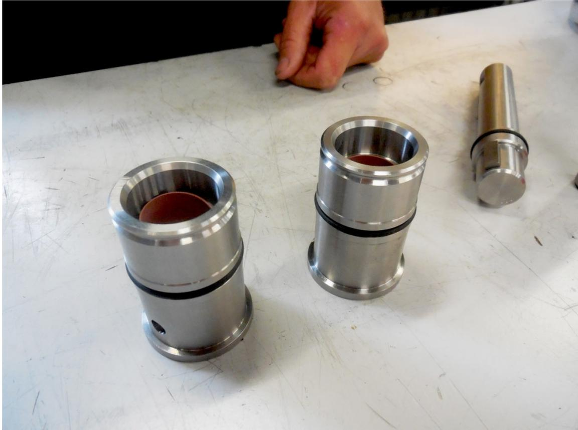
Firmly push down the Rulon bearing (KS-9) into the bearing sleeves (KS-4).
