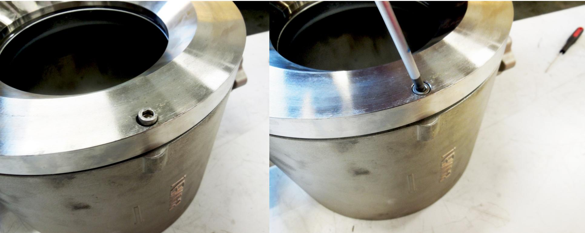
Secure the seat holding ring with two screws (KS-11)
