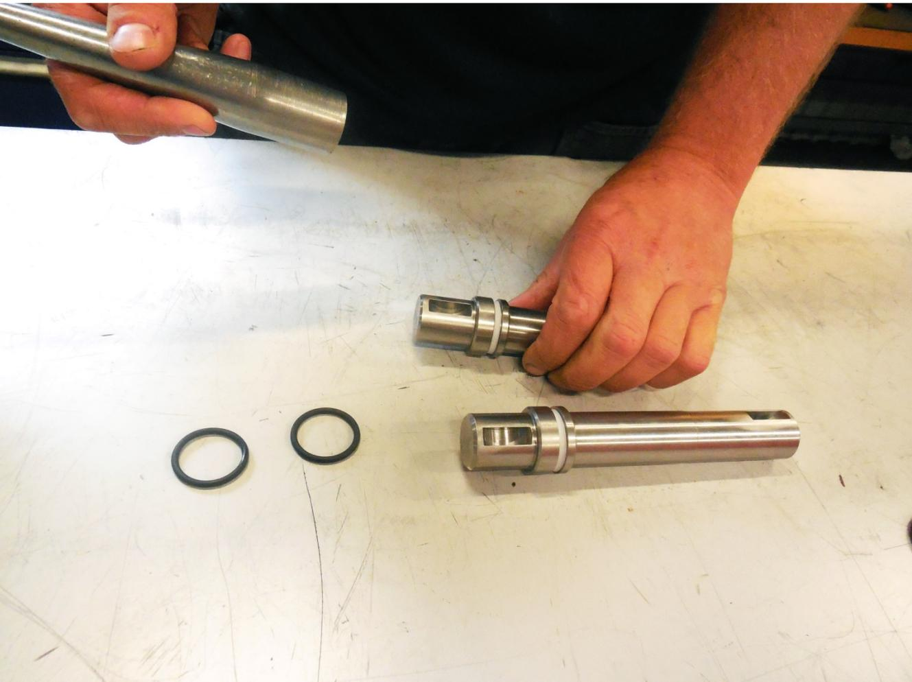
Mount the o-rings (KS-13) on the ball sector shafts (KS-5,-6) by using the special tool provided by Ramén.
