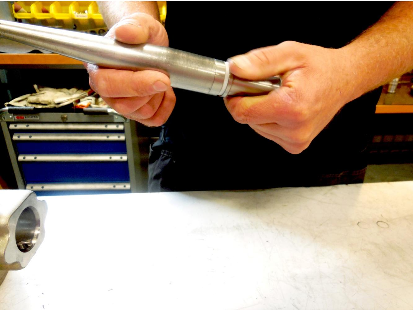
This is how the sliding rings (KS-13A) should look like when assembled on the shafts (KS-5,-6).
