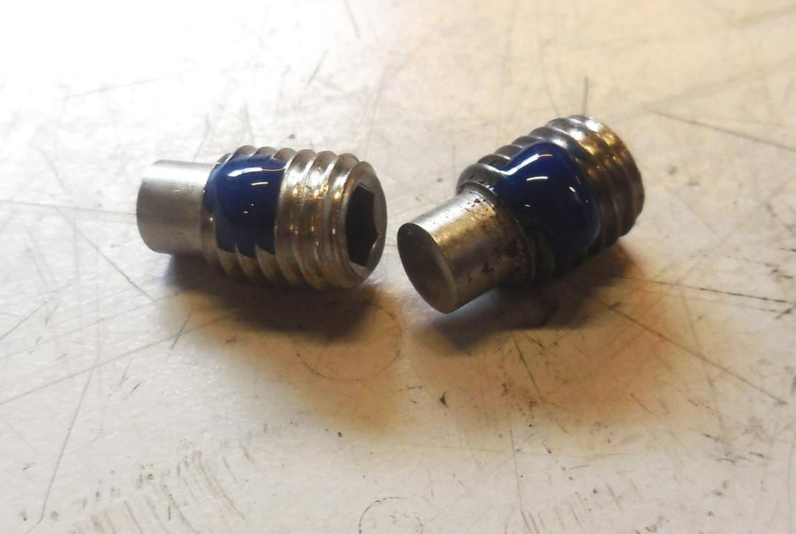
Use thread locker on both grub screws (KS-12).
