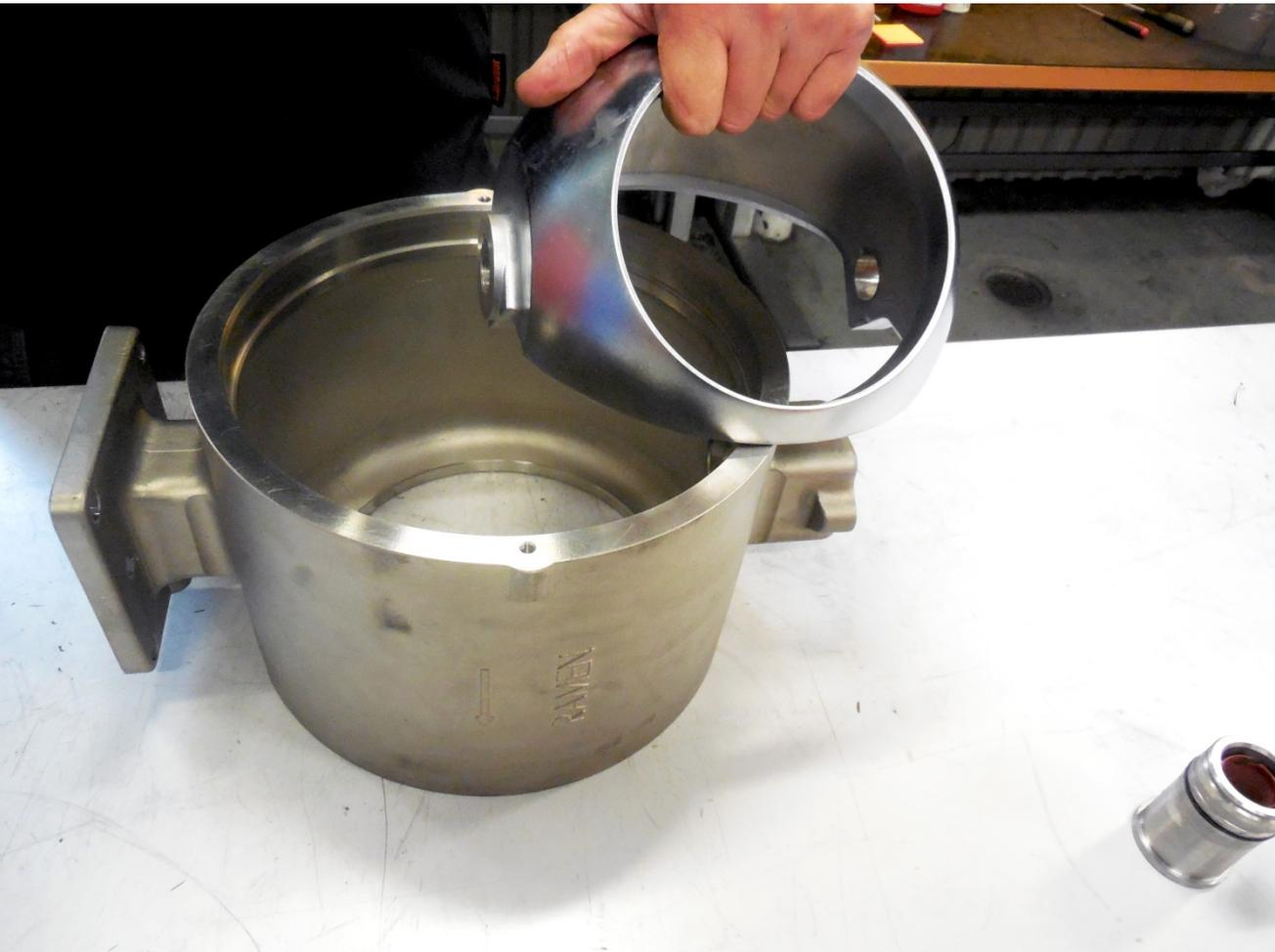
Put the ball sector (KS-3) into the body (KS-1), from the inlet side and with the seat sealing area positioned as shown in the picture.
