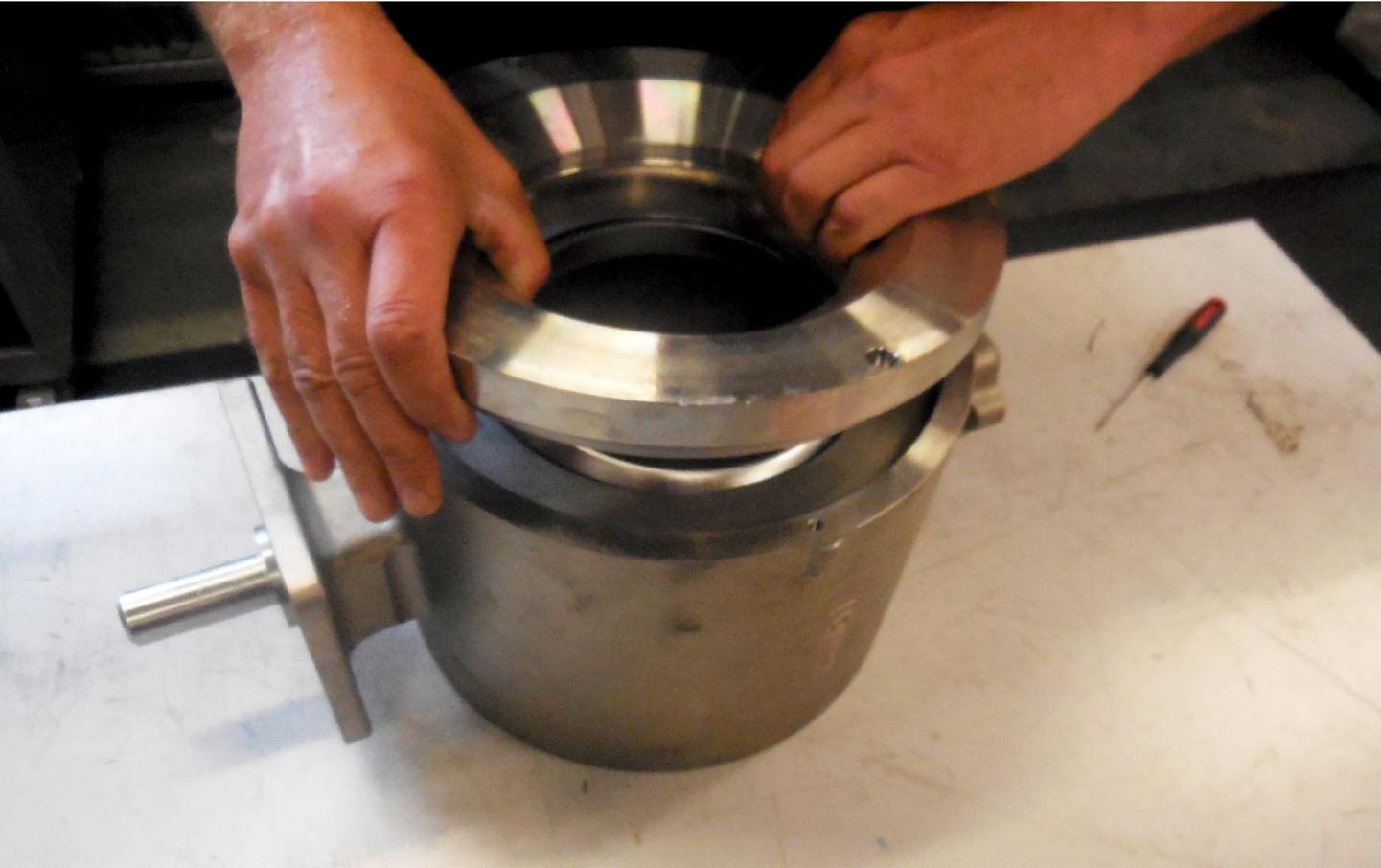
Assembly the seat holding ring together with the valve.
