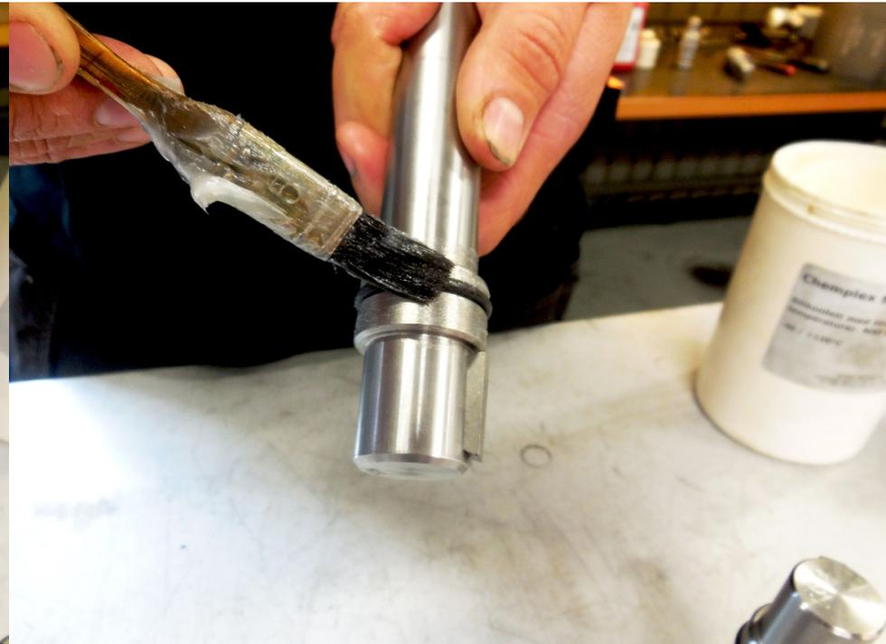
Apply generously of silicon grease, e.g. Chemplox SI 400M (Fuchs-Lubritech), with a brush on the O-rings assembled on the shafts and the bearing sleeves.
