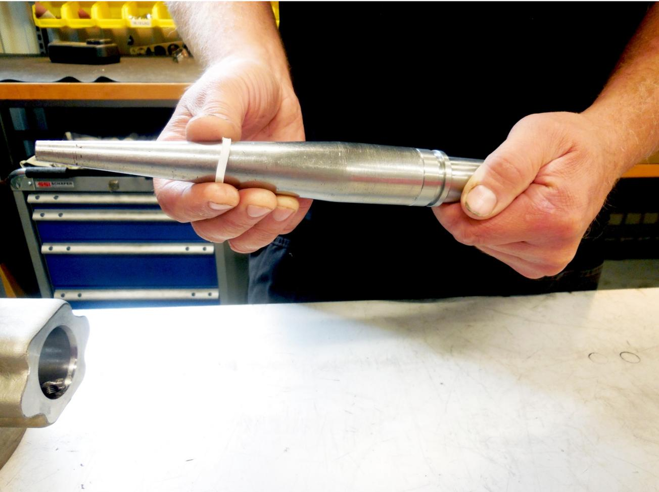
Mount the sliding rings (KS-13A) on the ball sector shafts (KS,-5-6) by using the special tool provided by Ramén. Preferably this should be done a couple of hours before assembling the O-ring.
