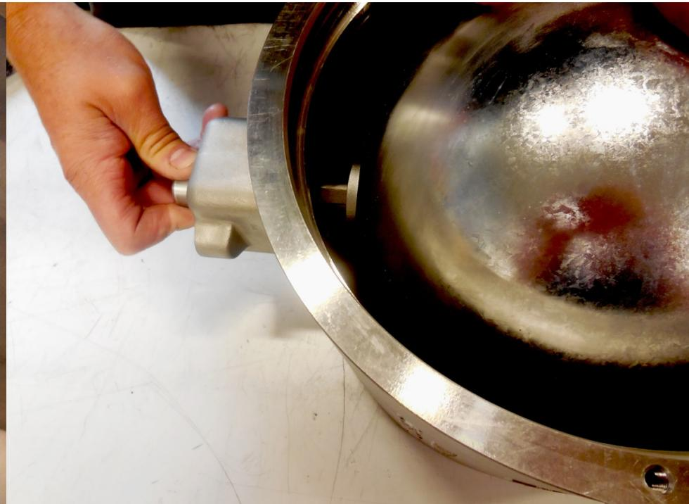
Assembly the short shaft (KS-5) in the body, aligning the ball.
