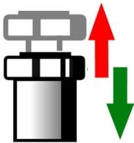
Step 1: Loosen the lifting knob and pull it upwards until blow-off of the operating medium is clearly audible.
