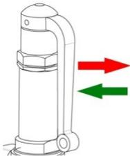
Step 1: Pull the lifting lever away from the spring cap until blow-off of the operating medium is clearly audible.
