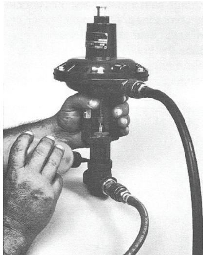
Figure 9: Pressure test the seals
