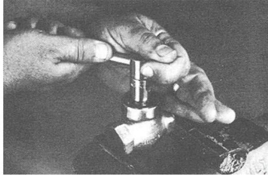
Figure 2: Unscrew the stem connector
