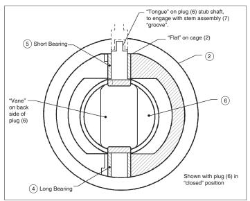
FIGURE 5 Back-end view of Cage/Plug Subassembly
