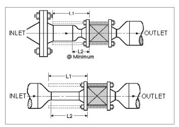
FIGURE 2: Line Bolting Clearance
