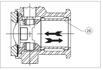
FIGURE 17 Reduced Trim Seal Retainer
