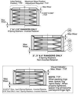
FIGURE 9 Ranger Live-Loaded Packing Design
