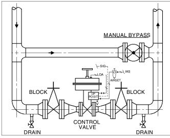
FIGURE 1: Typical Control Valve Station
