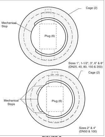
FIGURE 7 Mechanical Travel Stops - Plug in Closed Position Front-End View
