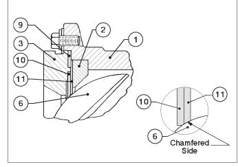
FIGURE 8: Typical Seal Assembly
