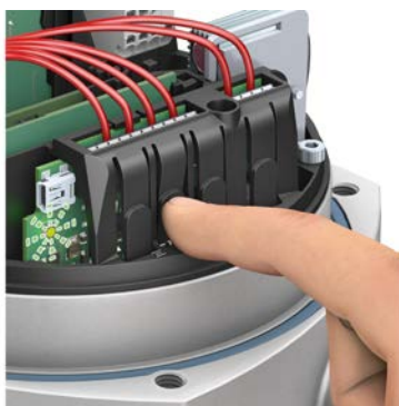
Figure 26: Operate in direction OPEN (example with I/O interface)
